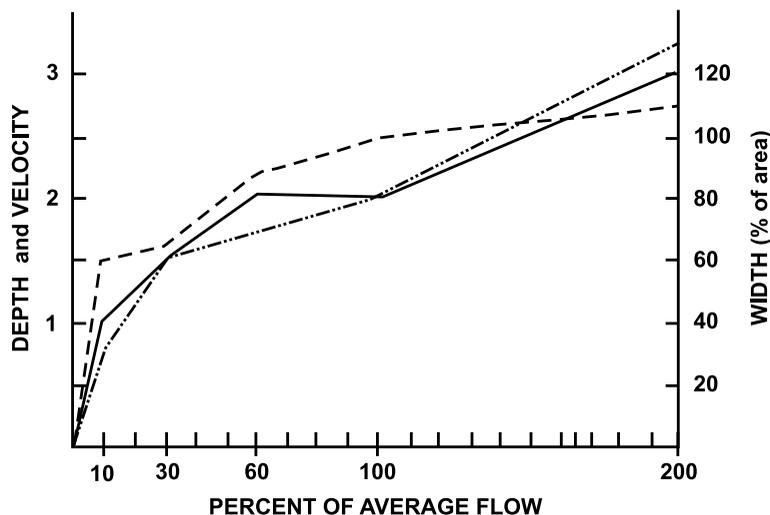
Figure 1. Relationship of flow (%) with channel width, depth and flow velocity (redrawn from Tennant 1976)
