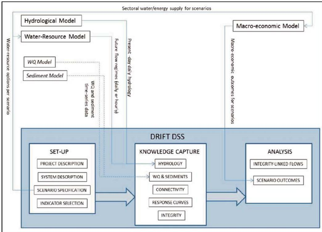
Figure 10. Arrangement of modules in the DRIFT-DSS and inputs required from external models (from Brown et al. 2013).
